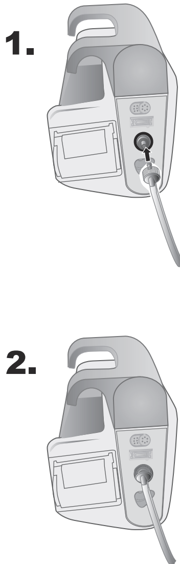
Figure 8-1 Attaching a Dual Lumen Hose to the Propaq MD Unit
