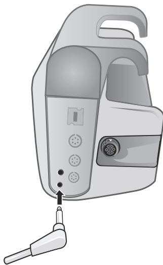
Figure 12-1 Connecting the Temperature Probe to the Propaq MD Unit
