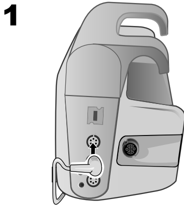
Figure 11-1 Plugging the Transducer into the Propaq MD Unit
