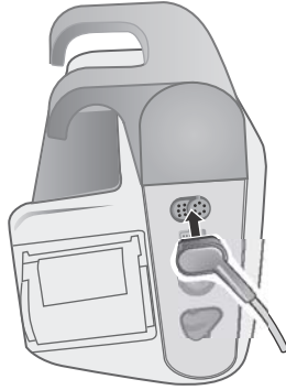
Figure 6-3 Connecting ECG Cable to Propaq MD Unit
