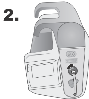
Figure 8-2 Attaching Single Lumen Hose to the Propaq MD Unit
