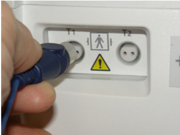
Figure 4.48. Temperature Probe Connections
