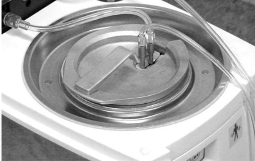
Figure 4.42. Replace the Cap on the Coolant Well
