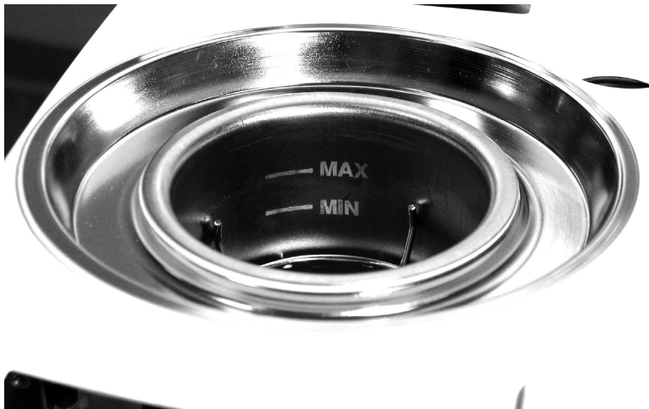
Figure 4.35. Coolant Well Liquid Level Indicator Lines
