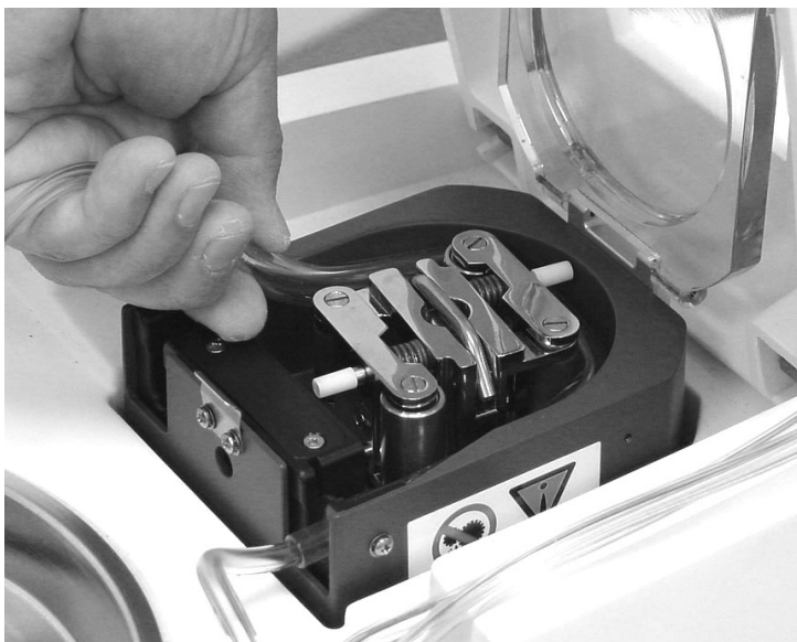
Figure 4.41. Pump Tubing Installation
