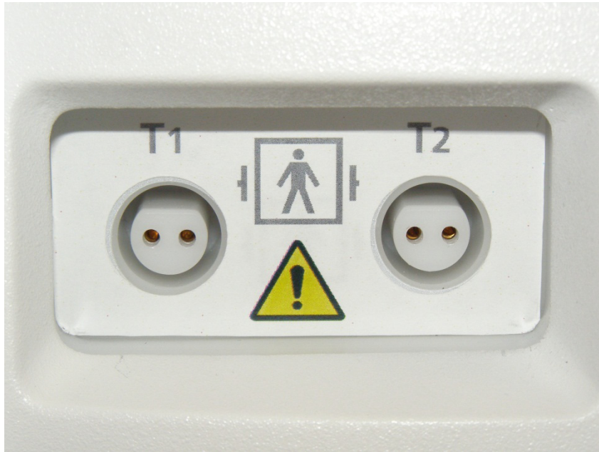
Figure 2.4. Temperature Probe Connectors.
