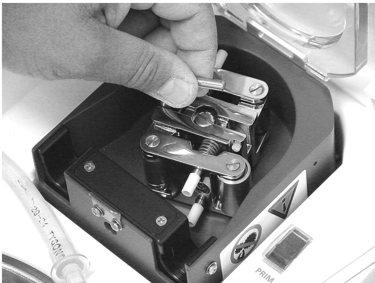
Figure 4.39. Lift the Pump Rollers Handle
