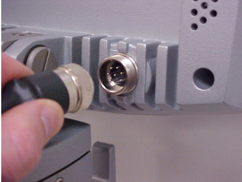
Figure 3.5. Plug the Control Cable Into the Socket
