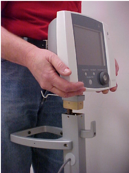
Figure 3.4. Attach the Display Head to the Mast
