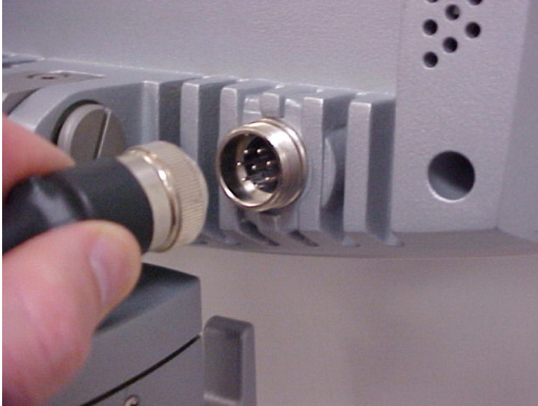
Figure 4.76. The Hirose Connector – Rear of the Display Head
