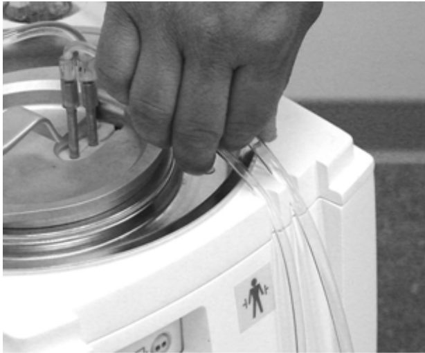
Figure 4.46. Route the Tubing Out of the Console
