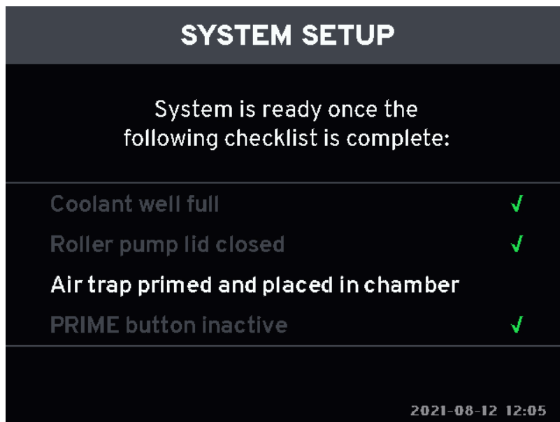
Figure 4.36. System setup checklist screen, Air trap primed and placed in chamber required
