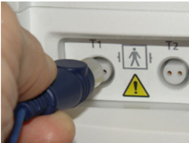
Figure 4.53. Temperature probe connections
