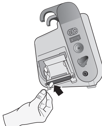
Figure 25-3. Cleaning the Print Head
